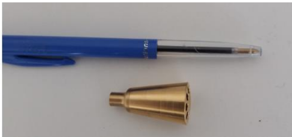
Figure 3: Picture of the distributor for 9 circuits
