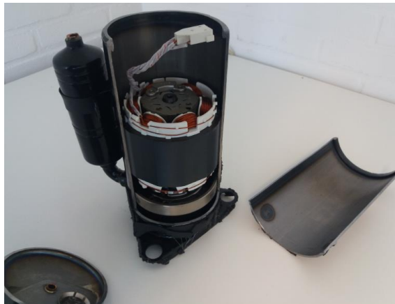
Figure 16: Large free volume exists above the motor within the shell of the GMCC DSM18019UDZ compressor.
