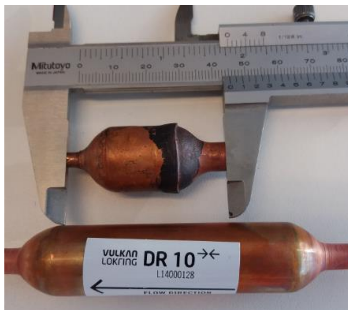
Figure 8: Picture of self-made filter. “The picture of the self-made filter is of a first trial in which a similar filter with a reduced outlet was modified. In the prototype the filters are of equal size but are made by modifying the Vulkan Lokring DR10 filter//drier”
